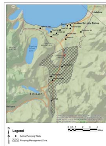
Proposed Pumping Management area which is based on simulated stream depletions in excess of 50 percent (from Pohl et al, 2018)
