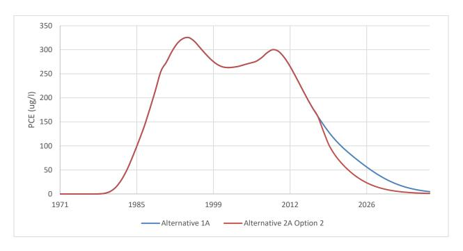
Figure 2. Simulated concentrations at the R1 site for the base (no-action) scenario (Alternative 1A), and Alternative 2A, option 2.
